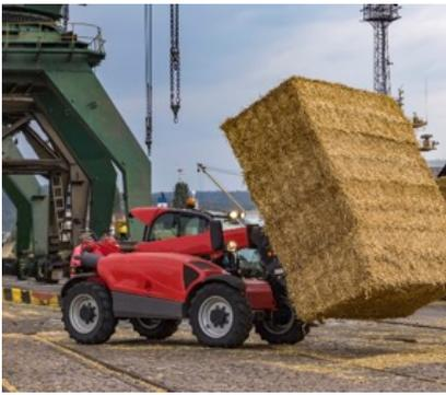
Stacking too high for the ability of the equipment (e.g. carrying five bales high instead of four).
