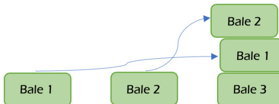
Figure 2: Less safe method of stacking bales – stack can become unstable
